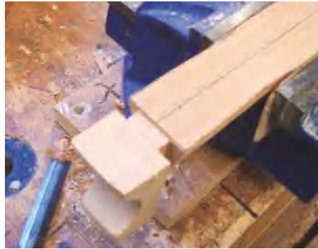
▲ Pic.21 The ledge to house the top of the soundboard
